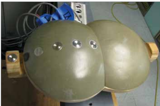
Figure 1. The REAR instrumented buttocks model showing pressure sensors
