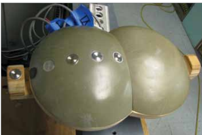
Figure 2. The ISO buttock model used for bench testing at The Rehabilitation Engineering and Applied Research Lab (REAR) at Georgia Tech University
