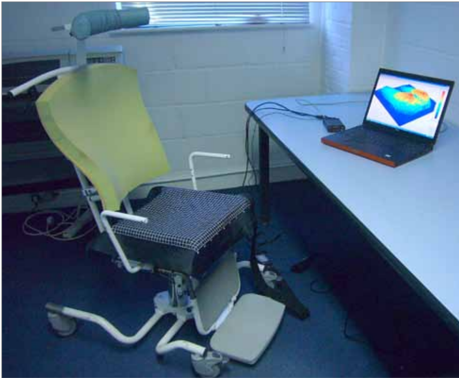
Figure 13. Test-rig and XSENSOR Pressure Imaging system
